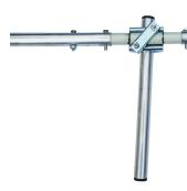
2. Fit the main elements onto the ends of the GRP rod and align the bolt holes. Insert the 2 outermost 35mm bolts and tighten the serrated nuts. The top main element section (with the end hat securing bolt) is on the right in the picture.
