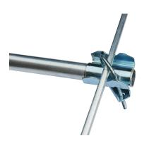
5. Attach the lower capacity hat element to the bottom of the lower main element using the second cross clamp as shown. Centralise the capacity hat element using the alignment marks and ensure it is parallel to the top element before tightening the clamp bolts. Fit the plastic end caps.
