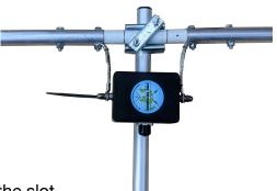
Slide the cable tie through the slot between the mounting block and the transformer housing and secure the assembly to the centre support arm. The second cable tie can be used for extra security or kept as a spare.
