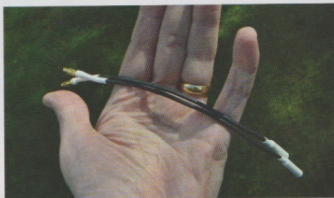
The antenna comes with an assorted of 'extenders' to move the resonant frequency down.
