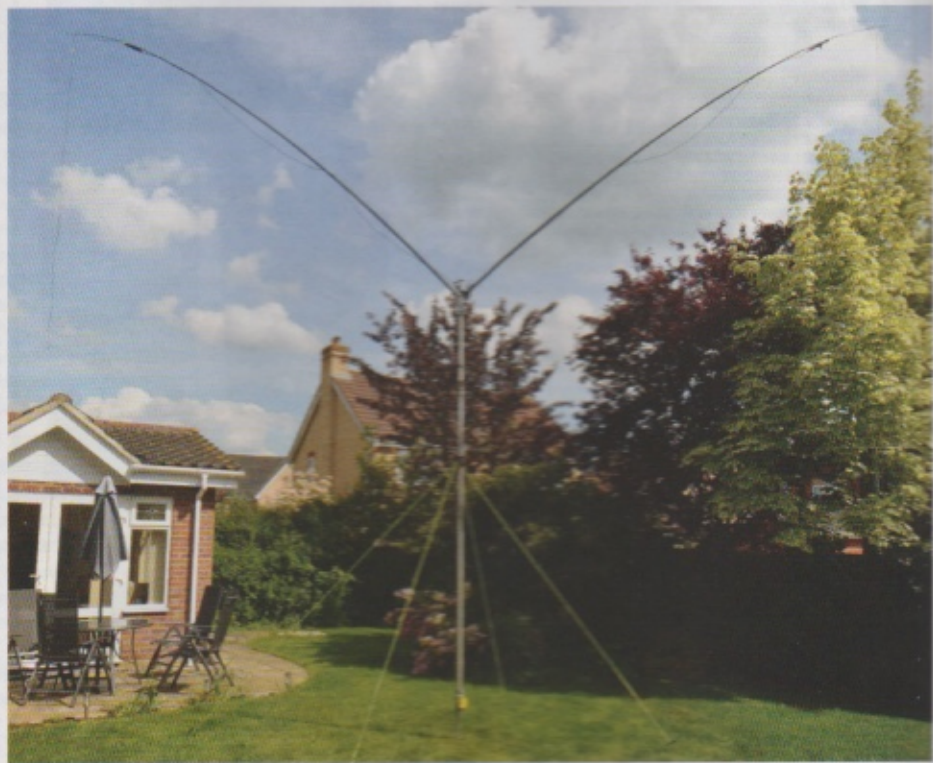
The DMV-II 80m antenna gets you onto 3.5MHz with a 'wingspan' of only about eight metres.
