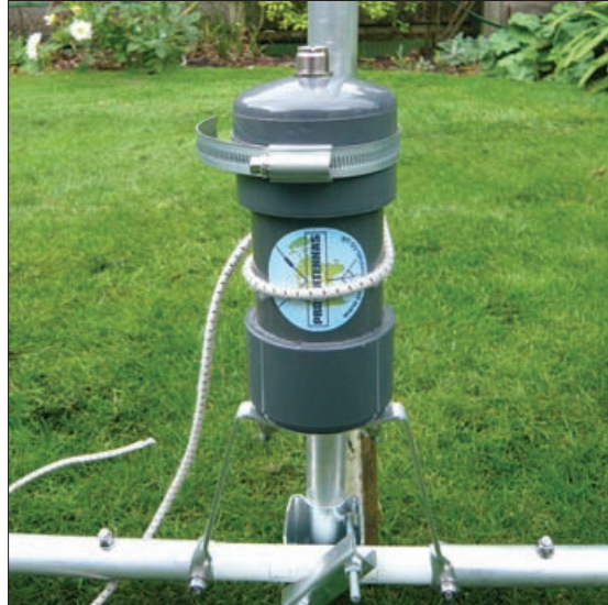
A close-up of the 'potted' balun.
